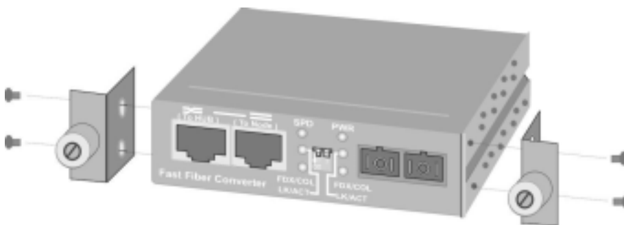
Figure 3-11. Attach rackmount ears on both sides of the modular converter
