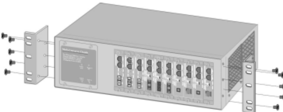
Figure 4-1: Attaching Mounting Brackets
