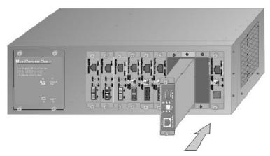
E. Gently push the thumbscrews in and turn clockwise to tighten. Do not over tighten the thumbscrews.
