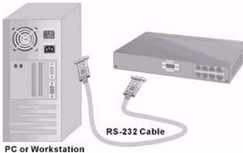
Connecting the switch to a terminal via RS-232 cable
