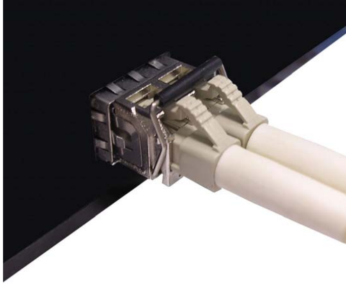
LC connector to the transceiver
